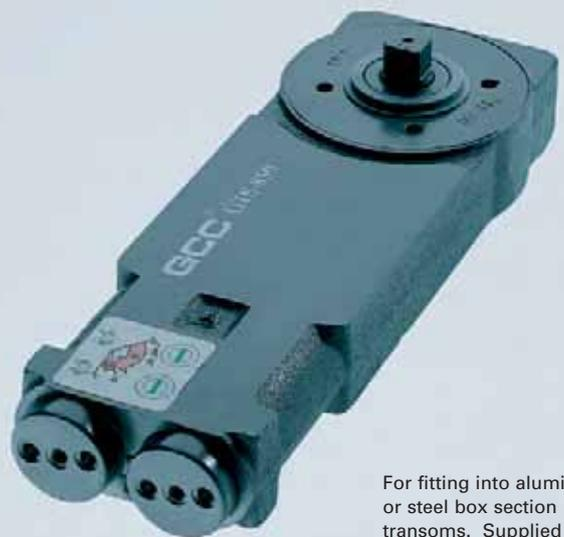
For fitting into aluminum or steel box section transoms. Supplied with 90° hold open facility as standard and the closing speeds are adjustable with valve no.1 operating from 130° to 20° and valve no.2 from 20° to centre.
